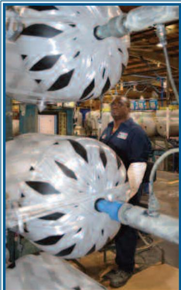
Highly trained technicians oversee H2PL tank winding being done on Flexcon's state-of-the-art automated filament winder.
