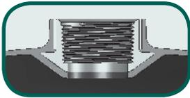
Top connections are encapsulated in precision molded domes to withstand the harshest environments.
